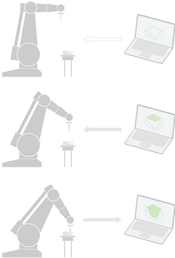
7 Once a rough approximation of a physical form is digitally modeled (top), the pipeline sends a point coordinate for the robot to move (middle). When touching, the smart pen sends analog sensor readings to through the pipeline over radio frequency (RF). A command is triggered to record and sent the robot's current world position the CAD file over Open Sound Control (OSC) (bottom) (Gannon 2014).
