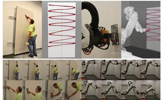
5 Skill Transfer from Trained Plasterer to MOCAP Tracking to Robotic Motion (Bard 2014)
