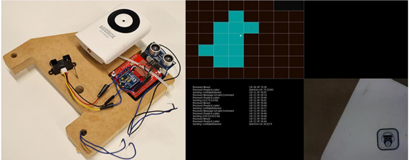
8 (left) Tool Prototype with Camera and Depth Sensor. (right) Grid Cell Search for Stock Definition and Refined Center (Jeffers 2014)
