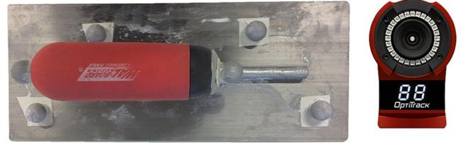
4 Plastering Trowel with Infrared Reflectors for Tracking (Bard 2014)
