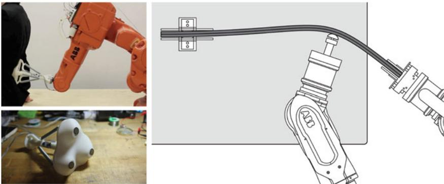
Fig. 6 Custom forming tool gauges pressure feedback from stressed wood
