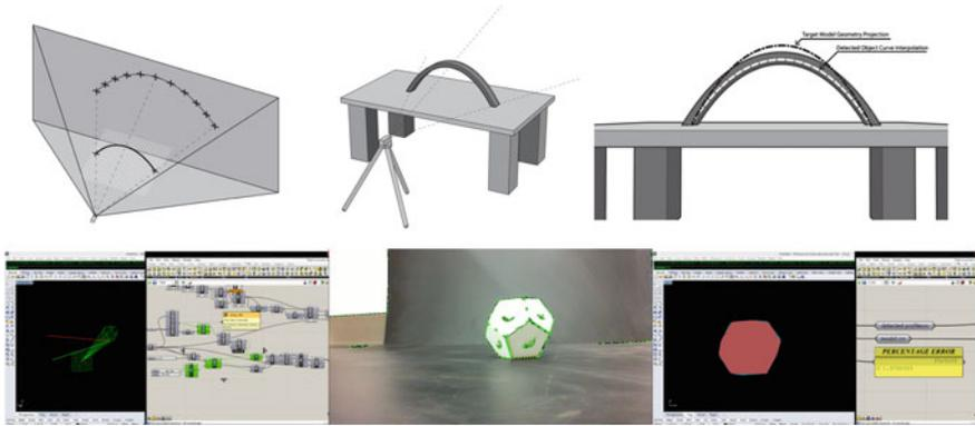
Fig. 5 Left digitally project desired curve. Center capture outline of physical bend. Right compare desired curve with physical bend and update motion
