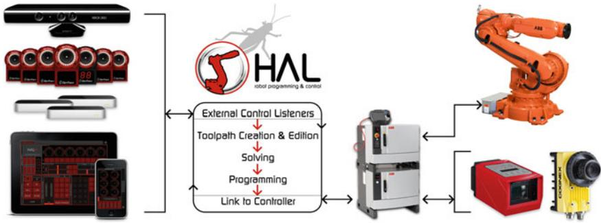
Fig. 3 HAL software architecture, in relation to external sensors and robot controllers
