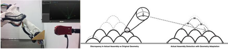
Fig. 7 Left calibrating motion capture and robot path. Right markers placed on physical components map the deviation between digital model and physical assembly
